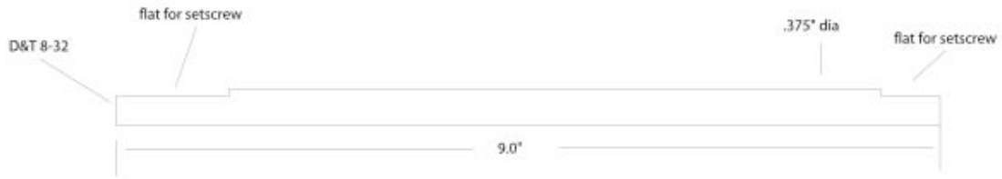
Figure 4: Stud shaft extension
